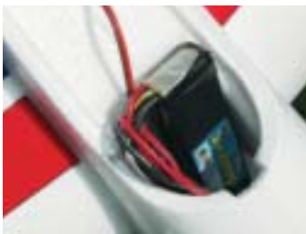
The Venom 3S 2200mAh pack nestles neatly into the fuselage and provides plenty of power for the AcroMaster.
