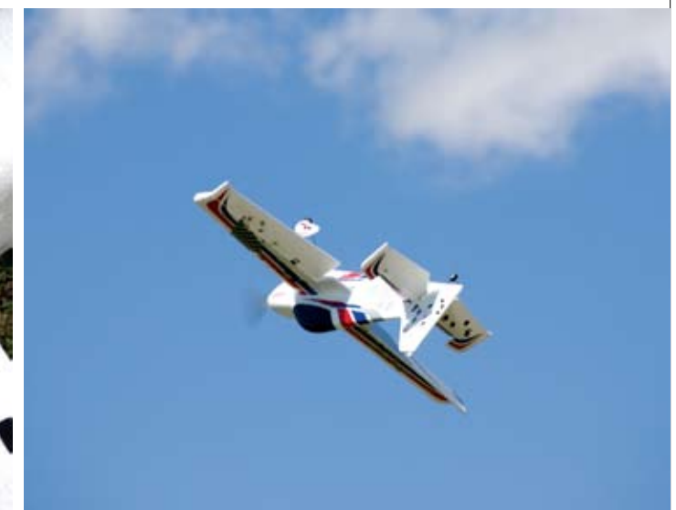
▼ Showing off the extreme control surface deflections with high-rates set for maximum throws! Tumbling and snapping maneuvers are very aggressive with high rates.
