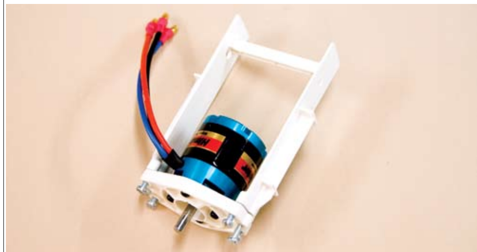
▲ The motor mount parts were bench-fitted to the motor to demonstrate how the parts fit together.
