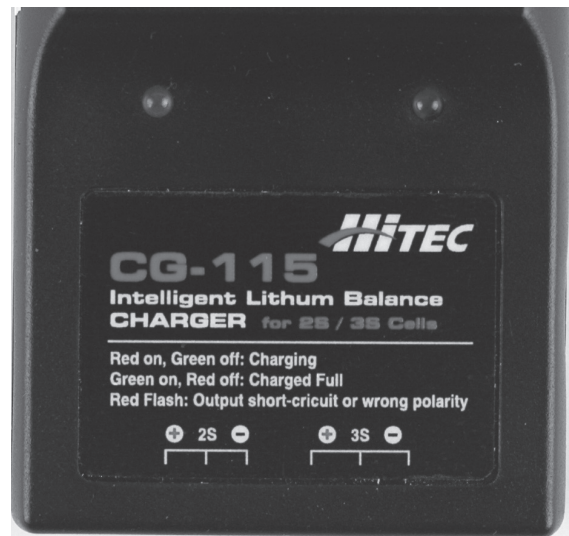
Charging information is printed on CG-115 Charger for reference
