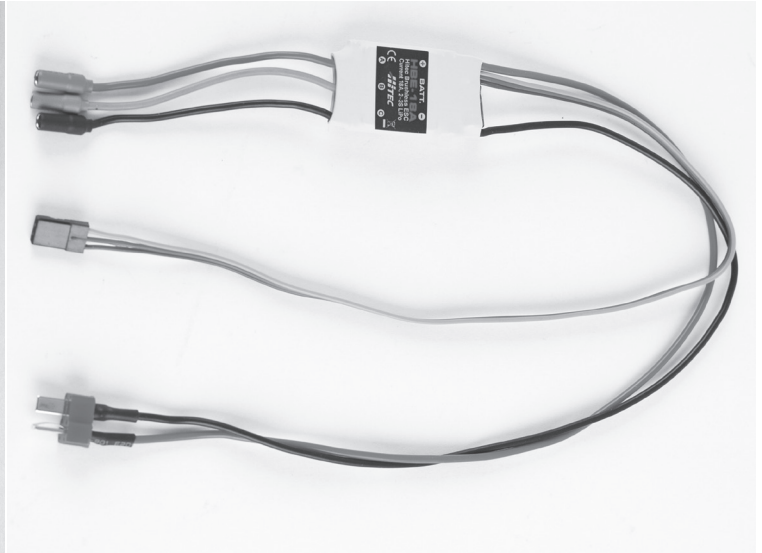
Hitec HBE-18AMP Electronic Speed Control showing (from top to bottom) connectors to the motor, receiver and flight battery.
