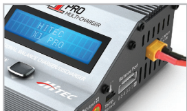
XT60 Connector plugged directly into charger
