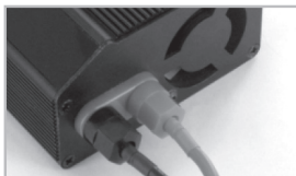
Bullet connectors plugged directly into power supply.
